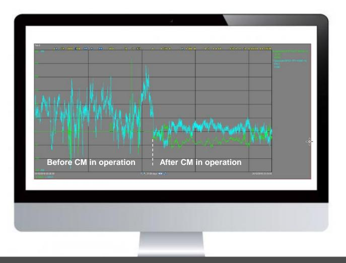
Dynamic voltage support during steady state and disturbances
